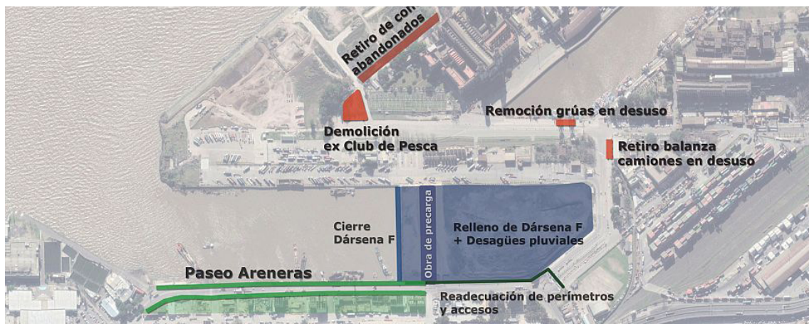
Containing works, backfilling, elimination of obstacles and development of pathways (completed or in progress) ©Puerto Buenos Aires
